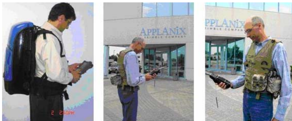
Figure 3. POS LS (left) and GPS-Denied Navigation and Mapping system (centre and right)
