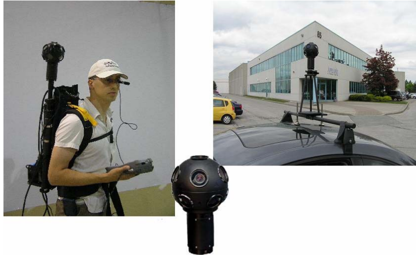
Figure 6. In-building mapping prototype: Backpack, camera and vehicle version.
